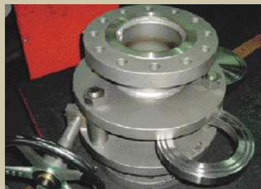
Step 3 turn the spectacle plate 90 degree
