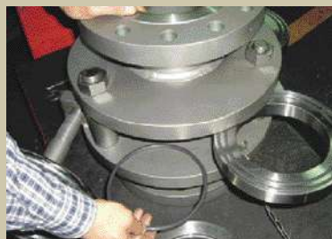
Step 5 replace the internal O-ring
