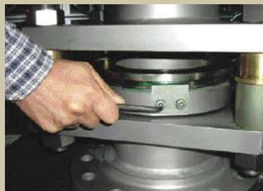
Step 3 remove the both seat holder
