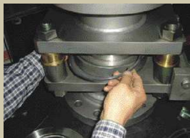
Step 5 replace the internal O-ring
