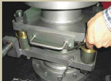
Step 1 remove the end-plate of the blind
